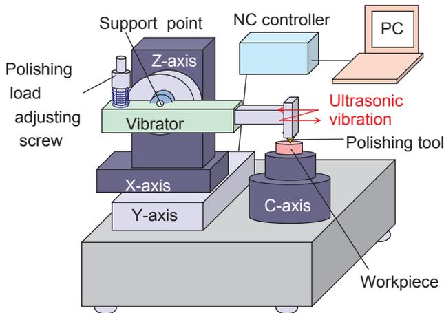
Figure 4: Schematic illustration of ultrasonic vibration assisted polishing machine.
