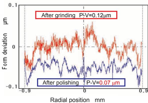
Figure 13: Form deviation profiles measured before and after polishing.
