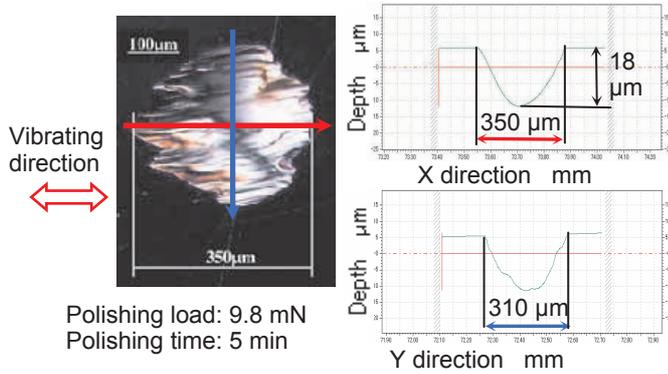
Figure 7: Shape of removal function.
