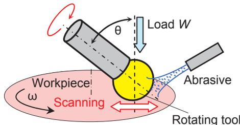
Figure 1: Conventional method with rotating polishing tool
