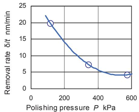
Figure 9: Relation between polishing pressure and removal rate.
