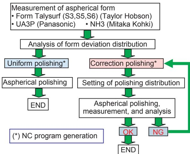
Figure 12: Flow chart of aspherical polishing process.
