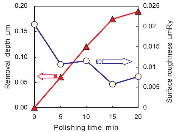
Figure 10: Changes in removal depth and surface roughness with polishing time.
