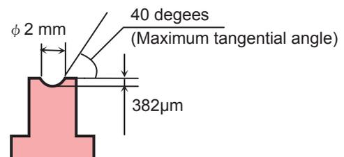
Figure 11: Geometry of workpiece for aspherical polishing.
