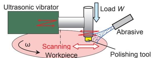
Figure 2: Proposed method with ultrasonic vibration assisted polishing tool.
