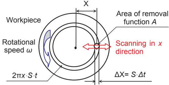
Figure 3: Polishing of axis-symmetric aspherical surface.
