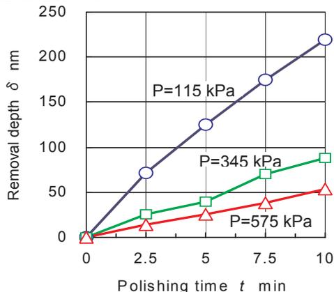
Figure 8: Change in removal depth with polishing time.
